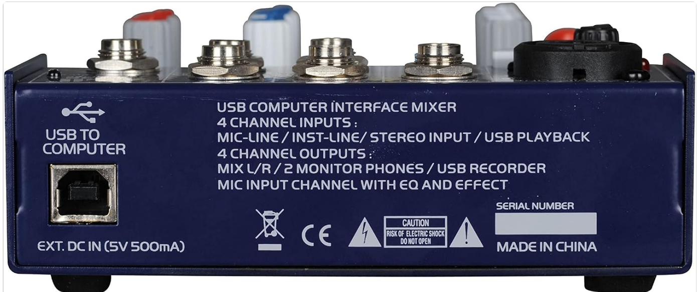
Figure 2: Rear view of the MUSYSIC MU-M4U mixer, highlighting the USB port for computer connection and the external DC power input.
