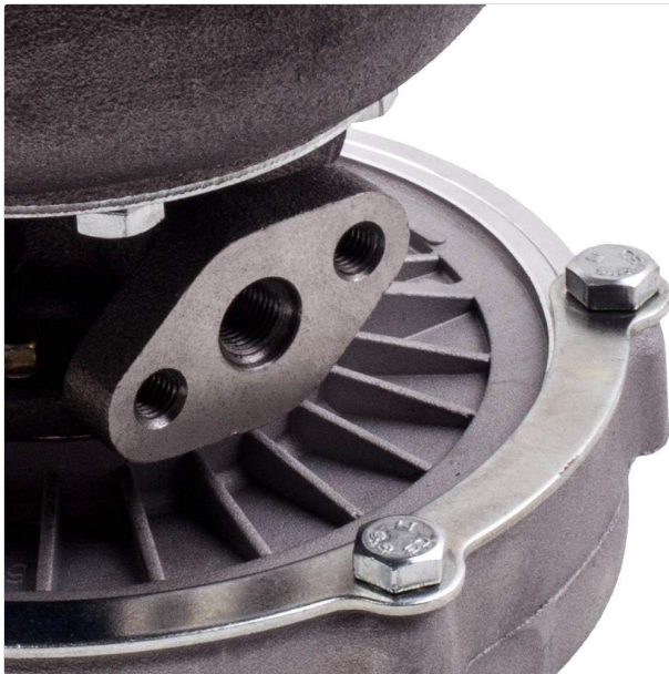
Figure 3.4: Close-up of the oil and water cooling ports.
