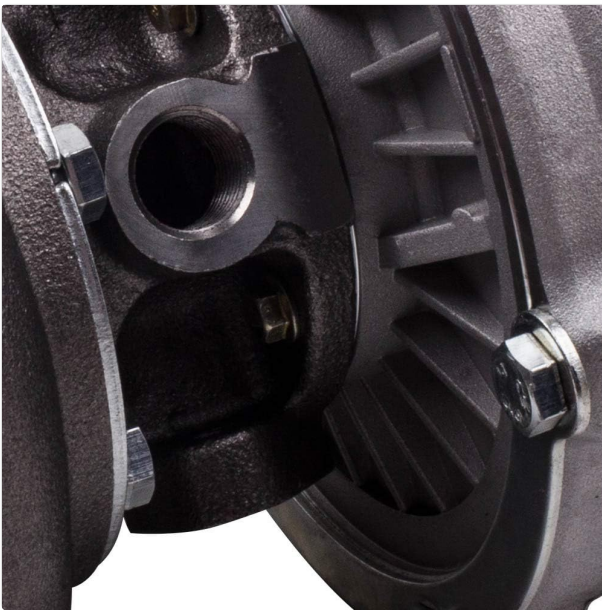
Figure 4.2: Close-up of the T3 standard exhaust inlet flange.
