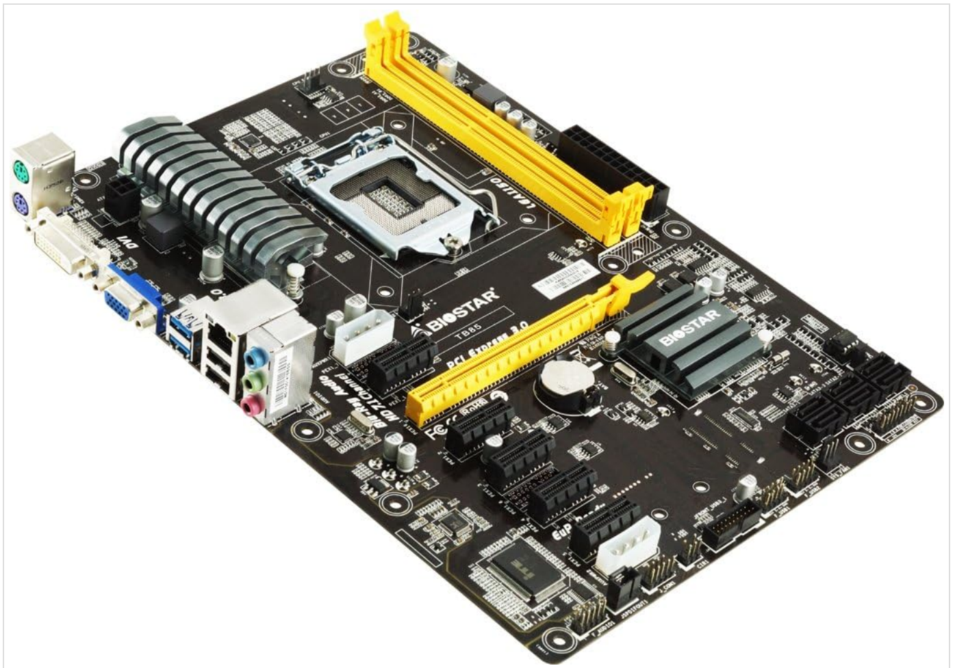
Figure 2: Biostar TB85 Motherboard Angled View. This image provides an angled perspective of the motherboard, showcasing the rear I/O panel with USB, audio, and video ports, as well as the CPU socket and the arrangement of PCI Express slots.
