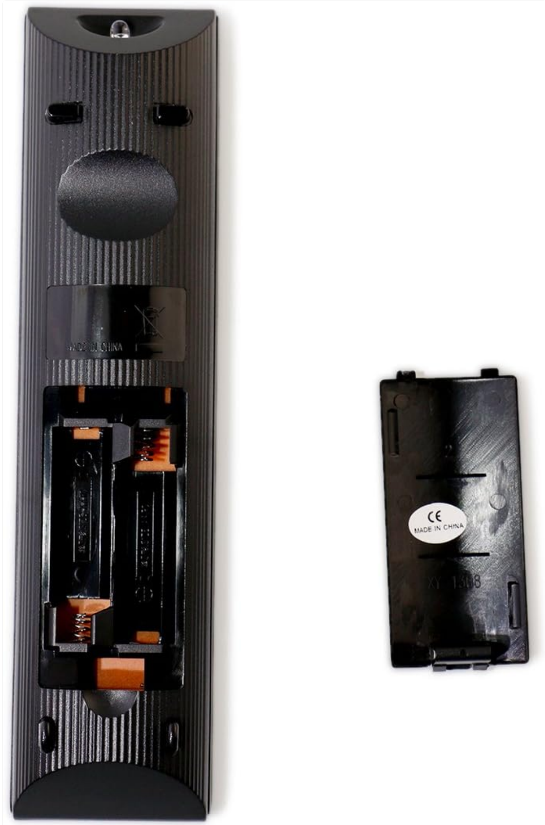
Image 2: Back of the remote control showing the open battery compartment and the detached battery cover, illustrating
