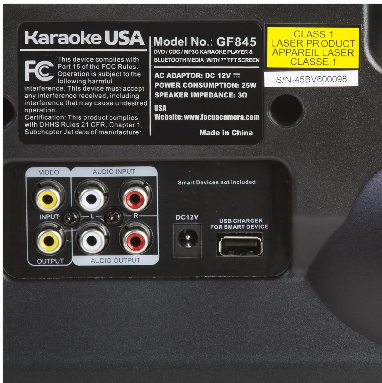
Figure 2: Rear panel connections, including DC 12V power input.
