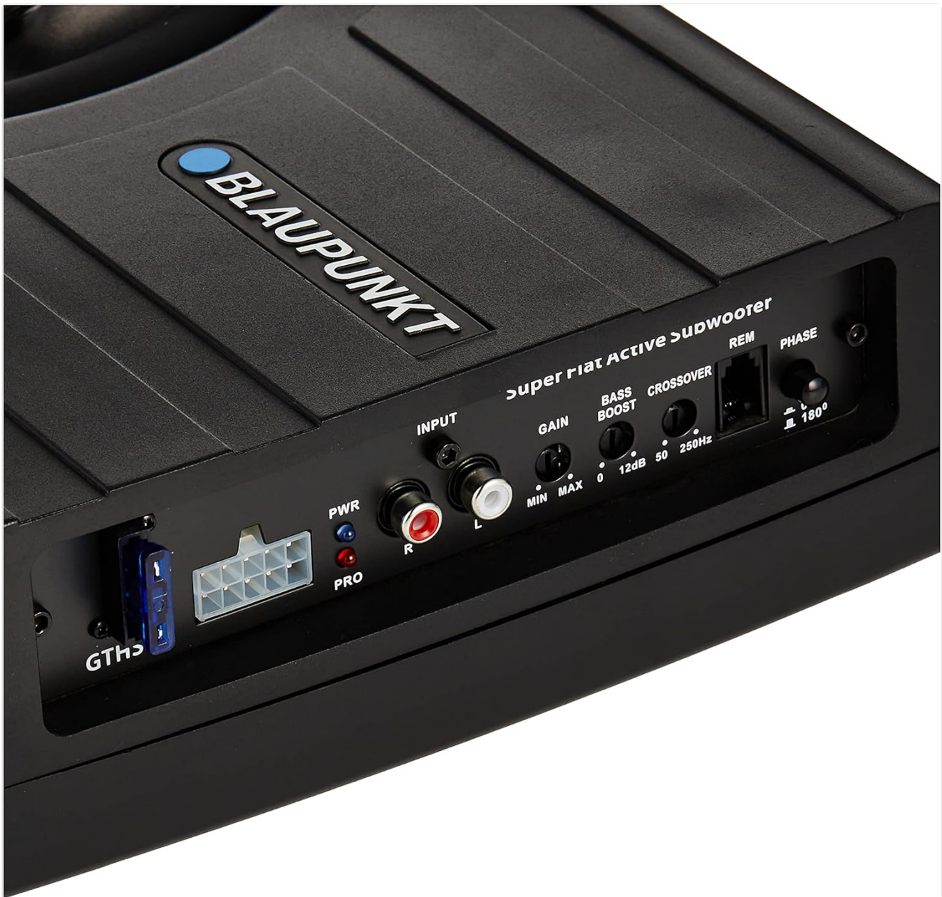
Figure 4.1: Control panel of the Blaupunkt GTHS80, showing power, input, and adjustment controls.
