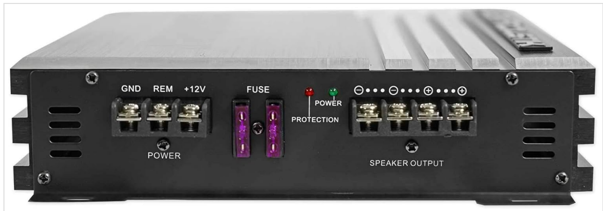
Image 4.2: Power input (GND, REM, +12V) and speaker output terminals on the amplifier.
