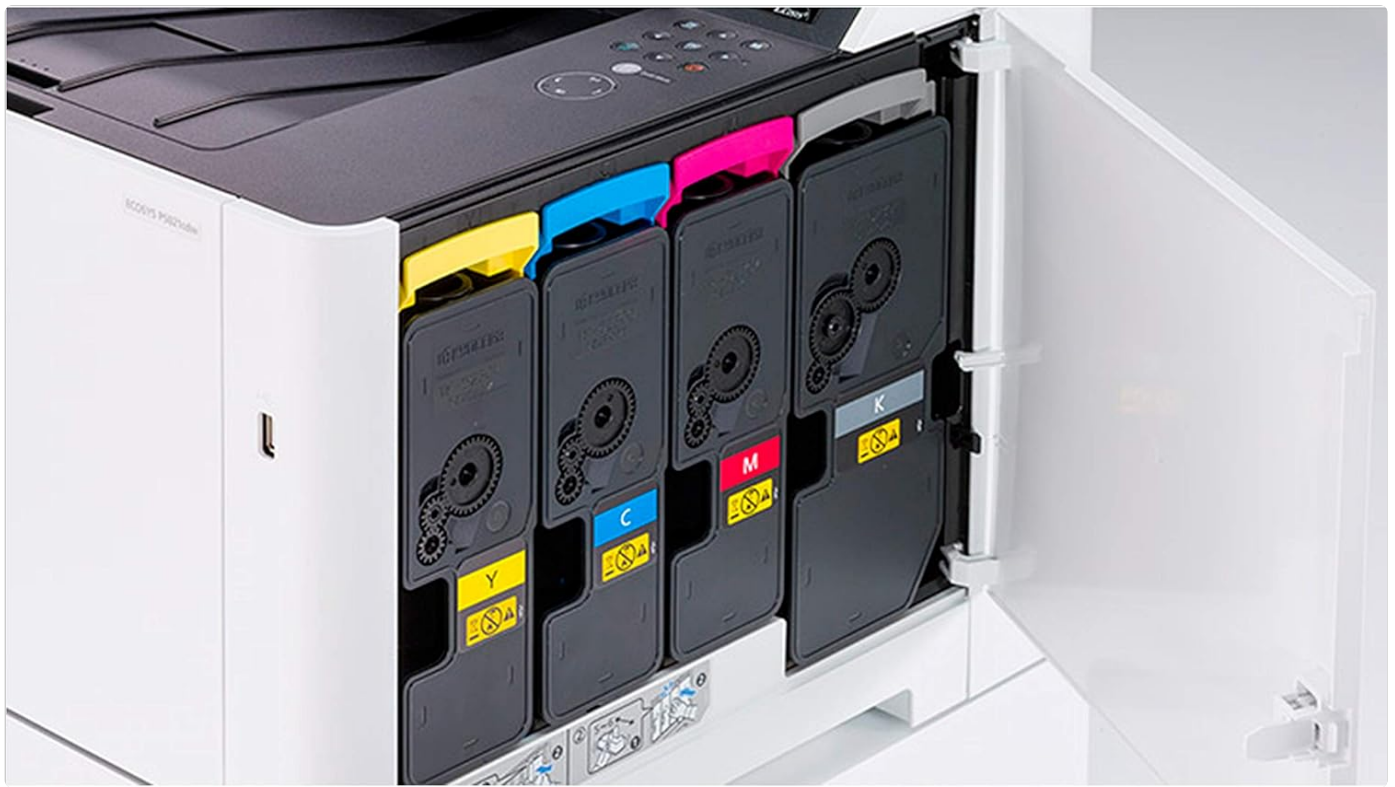
Figure 3: Close-up view of the toner cartridge installation area, showing the four color toner slots (Cyan, Magenta, Yellow, Black).
