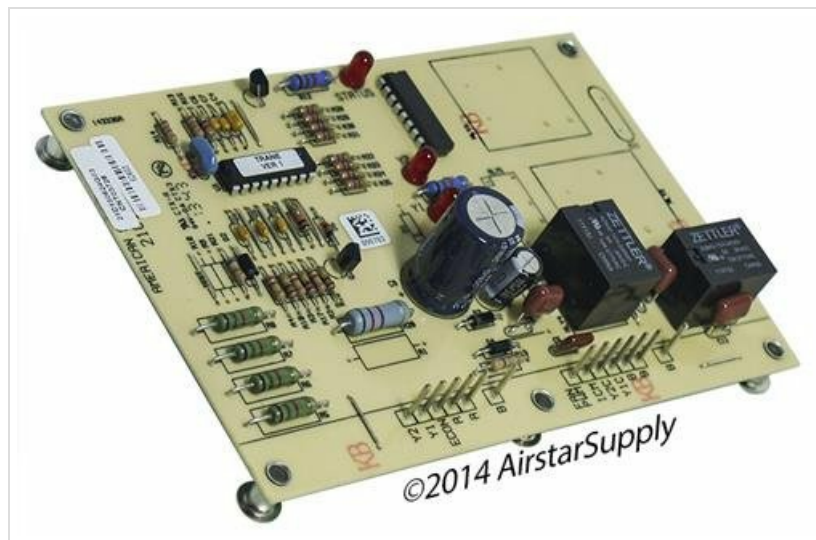
Figure 1: Angled view of the Trane CNT03728 Compressor Control Board. This image displays the overall layout of the circuit board, including integrated circuits, capacitors, resistors, and two prominent relays, along with various connection points.
