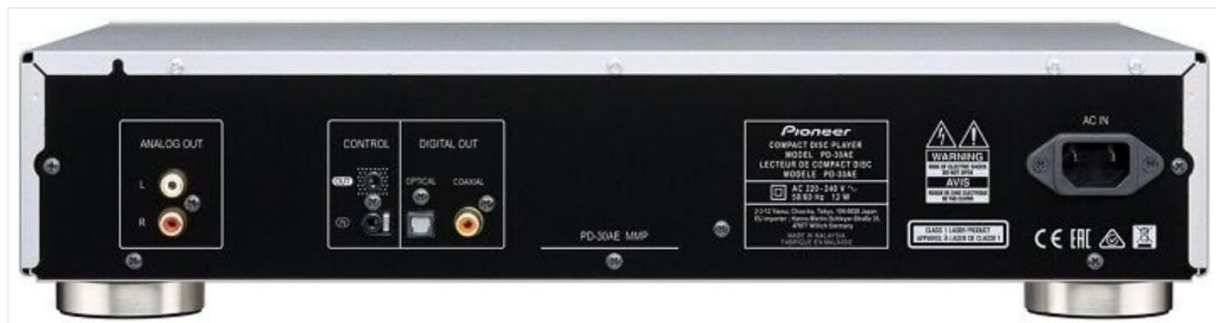
Figure 2: Rear view of the Pioneer PD-30AE CD Player, displaying the various input and output terminals. These include analog RCA outputs, digital optical and coaxial outputs, and the AC power inlet.
