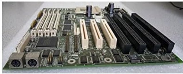
Figure 2: Angled view highlighting the PCI and ISA expansion slots, as well as the rear I/O ports.
