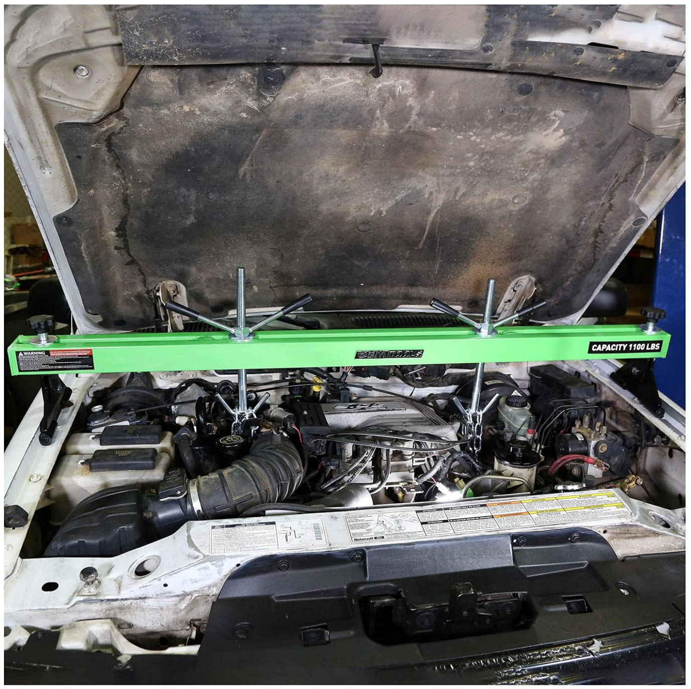
Figure 3.2: Top-down view of the engine support in operation, demonstrating how it straddles the engine bay to provide stable lifting points.
