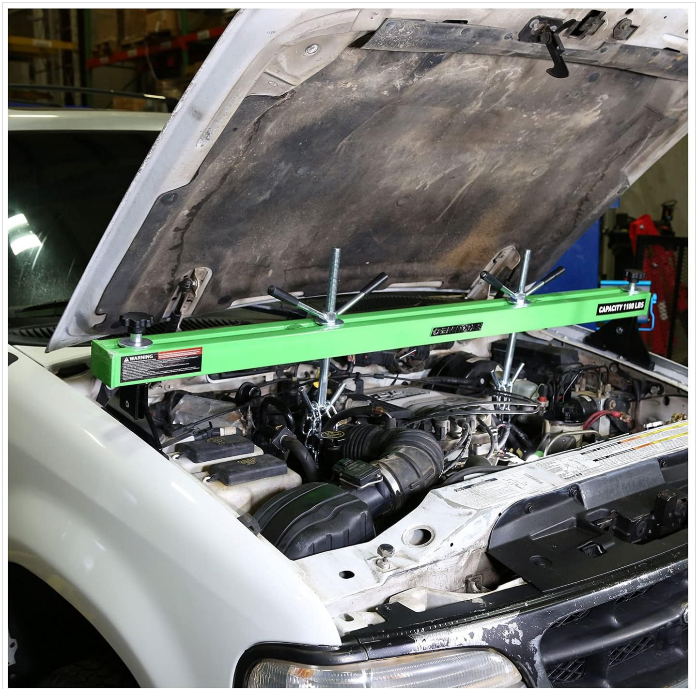
Figure 3.1: The engine support positioned across the fender wells of a vehicle, providing overhead support for engine work.
