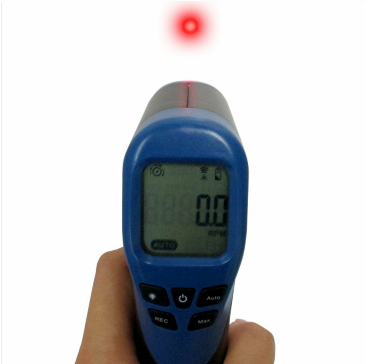
Figure 7: Laser Beam Emitting from Tachometer
