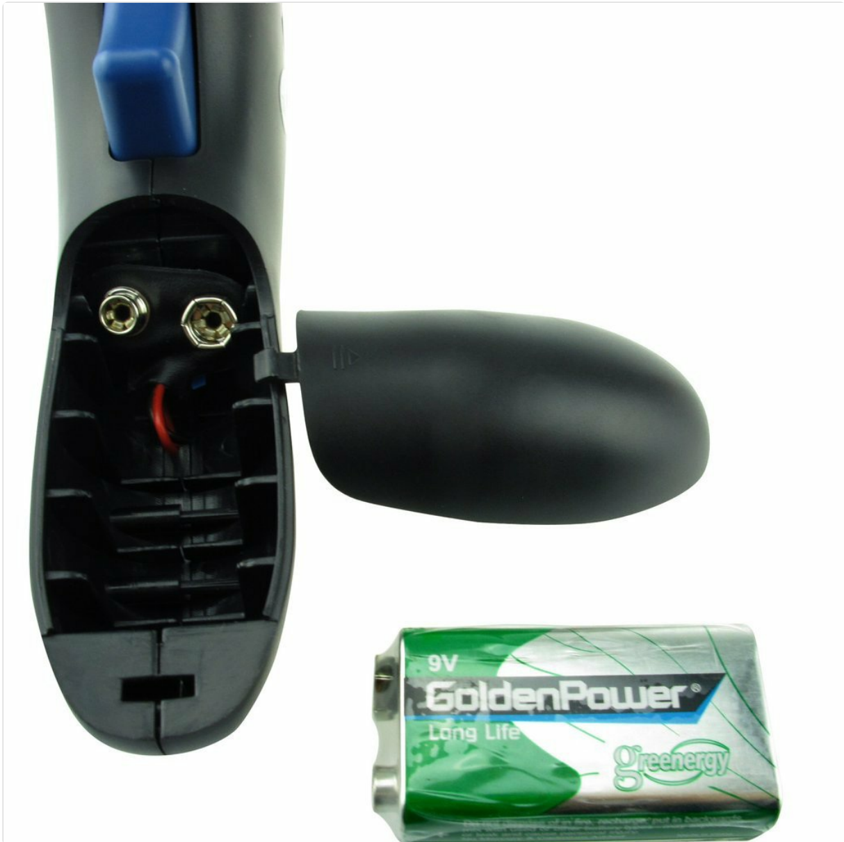
Figure 5: Battery Compartment and 9V Battery
