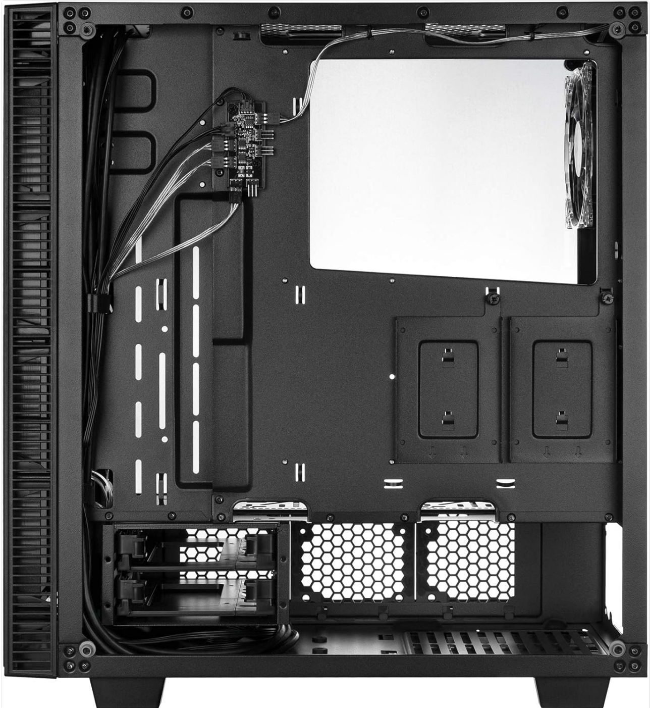
Figure 5: Rear interior view highlighting cable management options.
