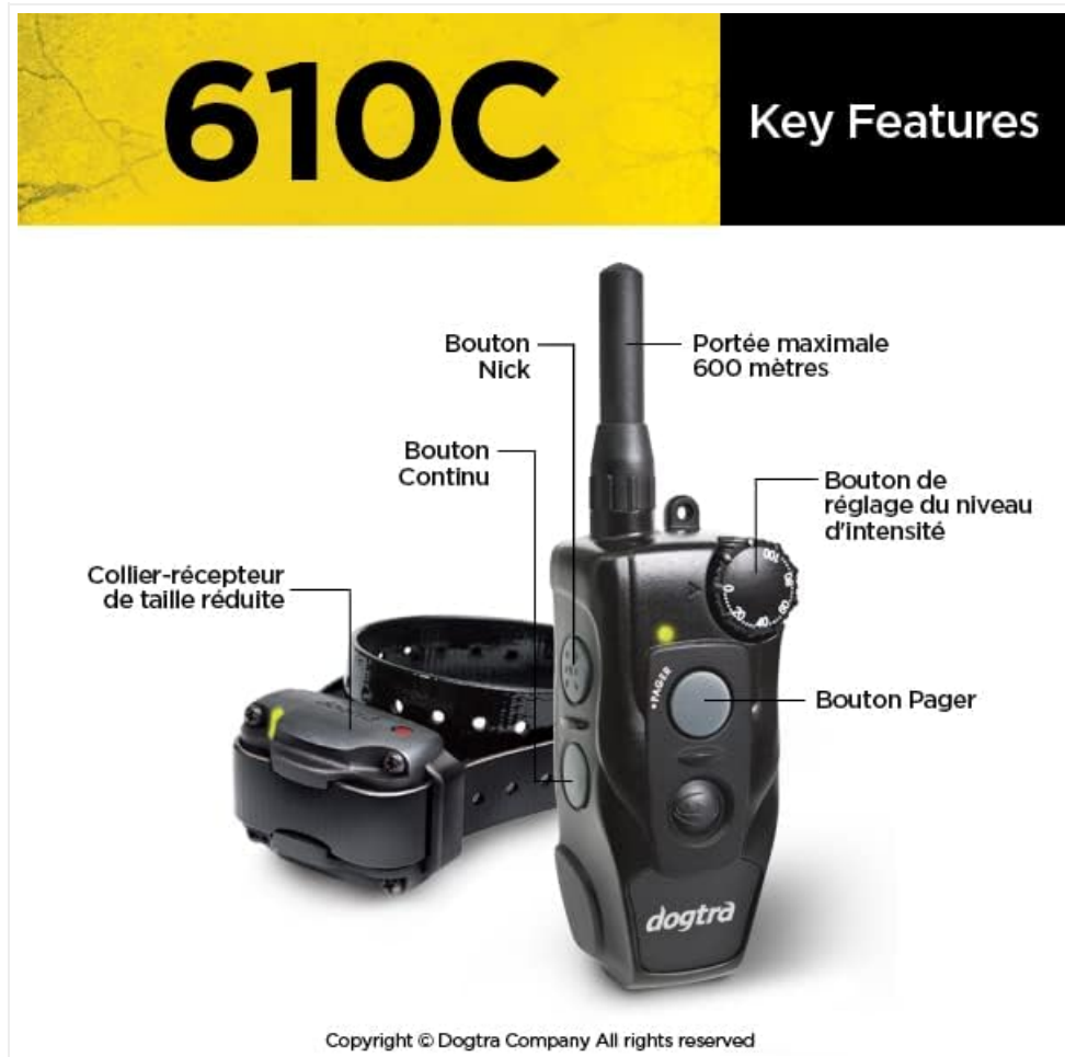
Image: Labeled diagram of the Dogtra 610C handheld transmitter, highlighting its controls.
