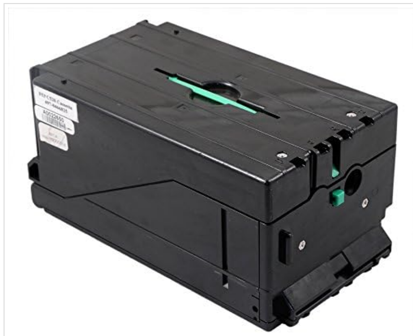
Figure 1: The Fujitsu KD03234-C520 Cash Cassette. This image shows the black rectangular cassette with a green lever visible on the top surface and a label on the left side indicating the model number.
