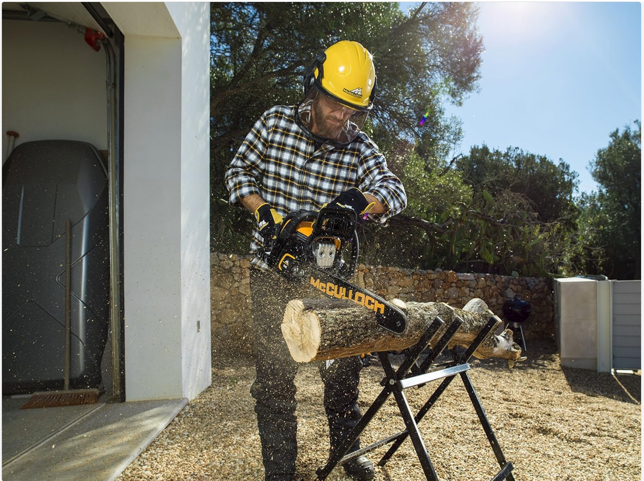
Figure 5.3: Close-up of an operator wearing full protective gear, including a helmet with face shield, while using the McCulloch CS 50S Chainsaw to cut wood.
