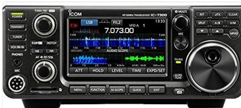
Figure 2: Close-up view of the Icom IC-7300's front panel, highlighting the large color display and control layout.
