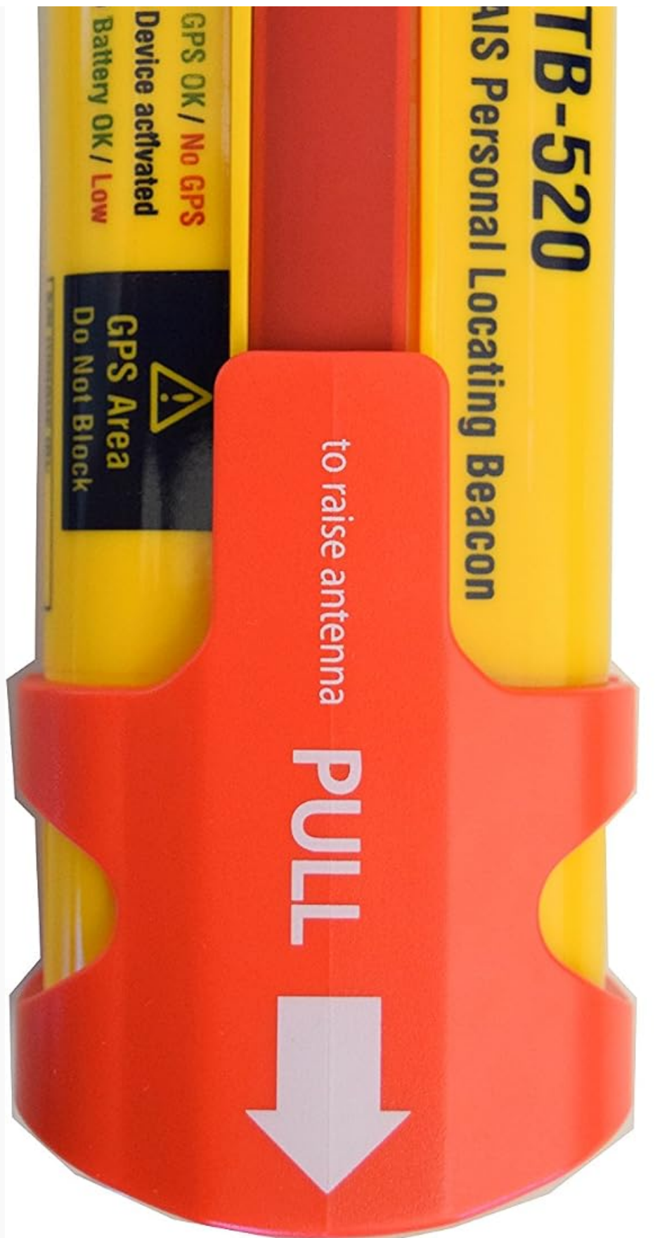
Figure 2.1: Front view of the AMEC TB-520 beacon, showing indicators for GPS status, battery level, and activation, along with the pull tab for antenna deployment.
