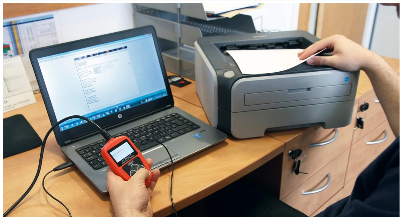
Figure 8: The BT105 connected to a laptop, demonstrating the print function for test results.
