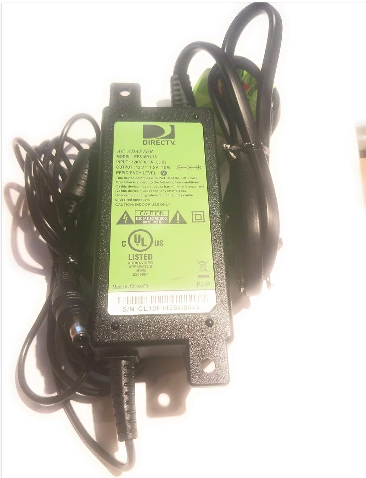
Image: The DIRECTV AC Adapter showing its label with electrical specifications (Model: EPS10R1-15, Output: 12V 1.5A 18W) and UL listing.
