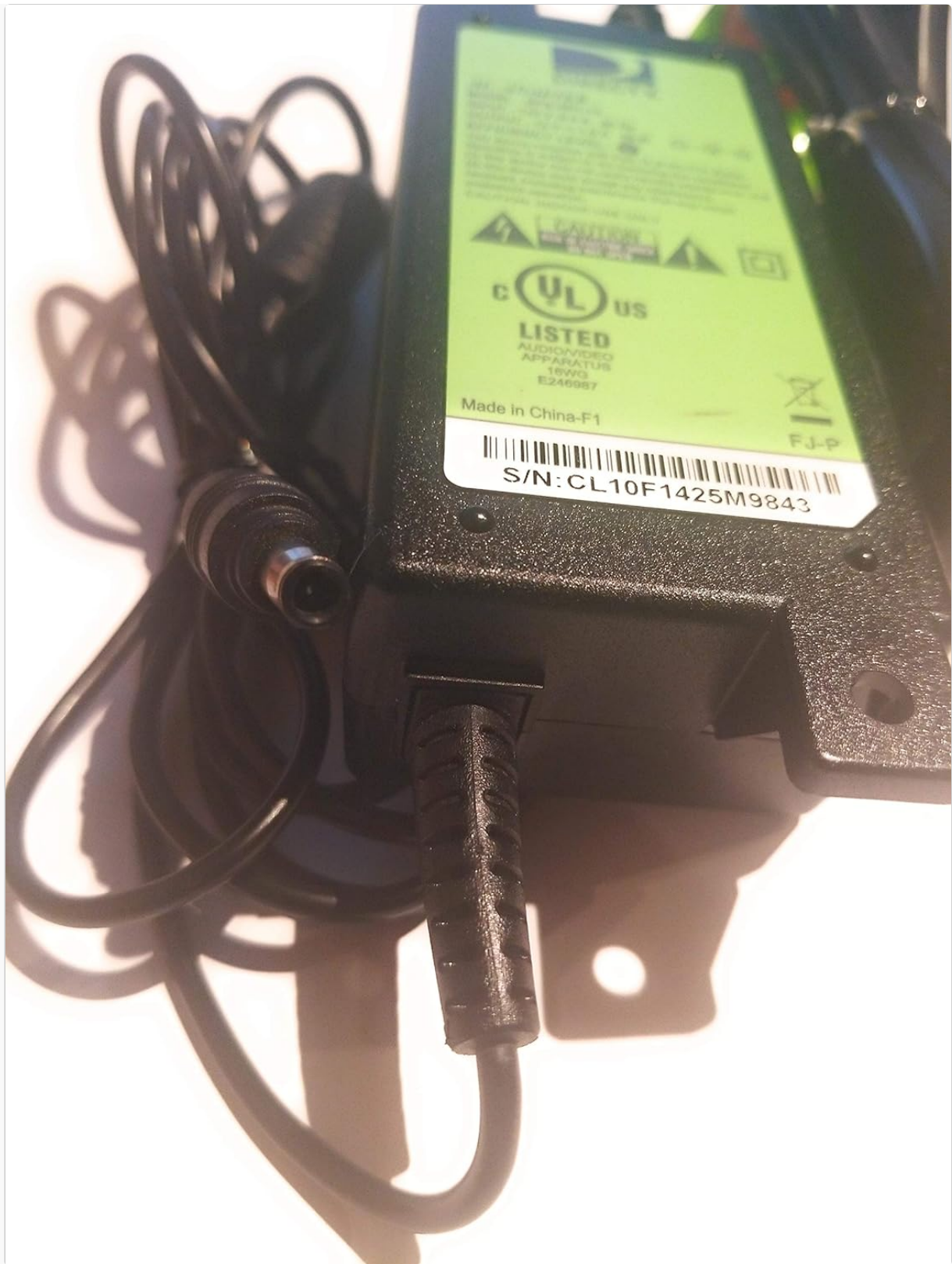
Image: Close-up view of the DC output barrel connector of the DIRECTV AC Adapter, ready for connection to a device.
