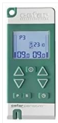
Figure 1: Cefar Peristim Pro Electrostimulator. This image shows the compact, handheld device with a green and white casing, a digital display, and control buttons for program selection and intensity adjustment.
