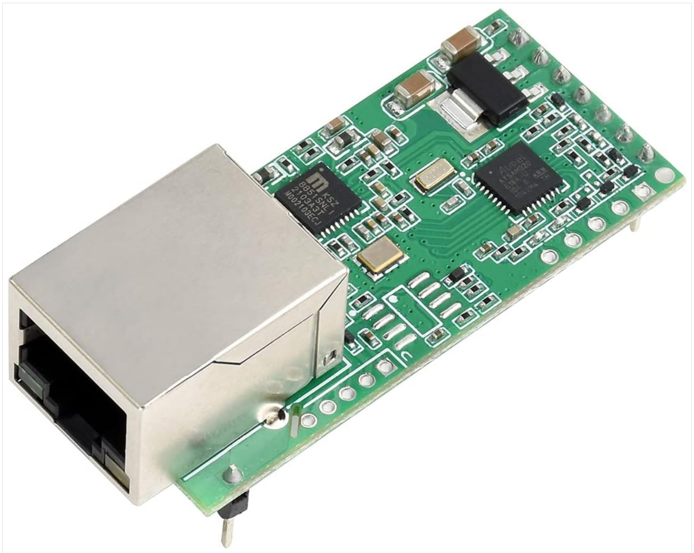
Figure 1.2: Angled view of the Waveshare UART to Ethernet Converter Module, highlighting the compact design and pin headers.
