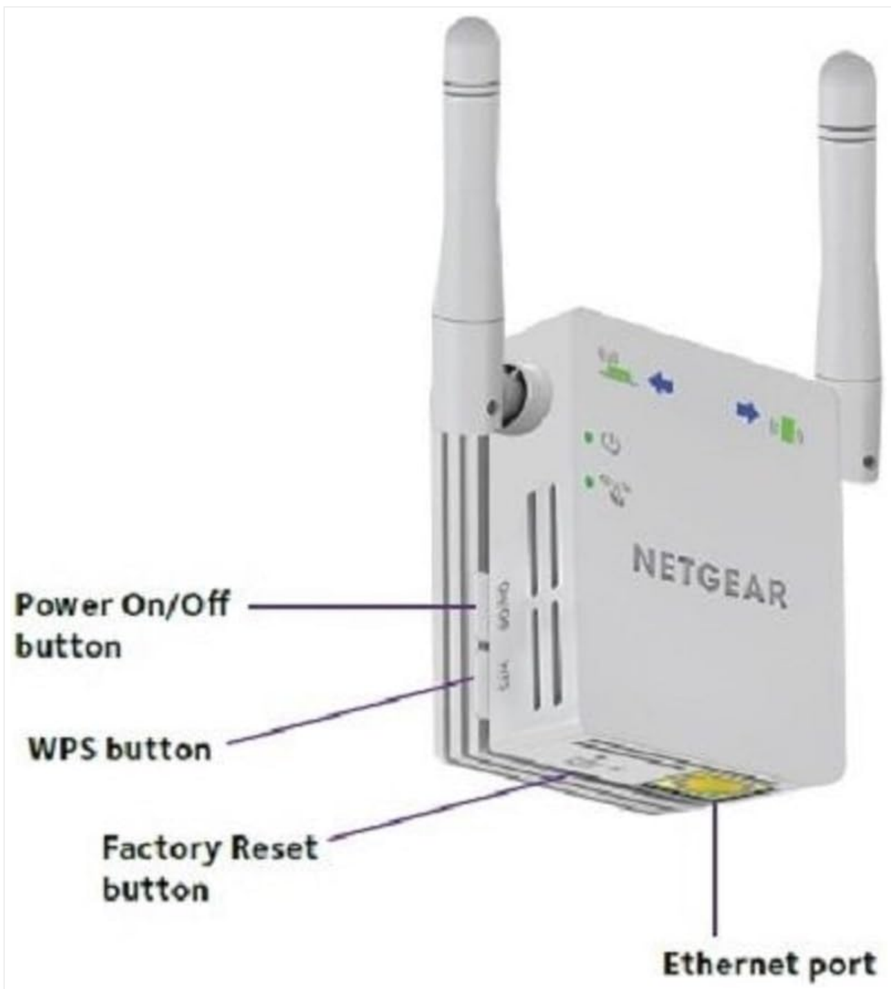
Figure 3.1: Side view of the extender, highlighting the Power On/Off button, WPS button, Factory Reset button, and Ethernet port.
