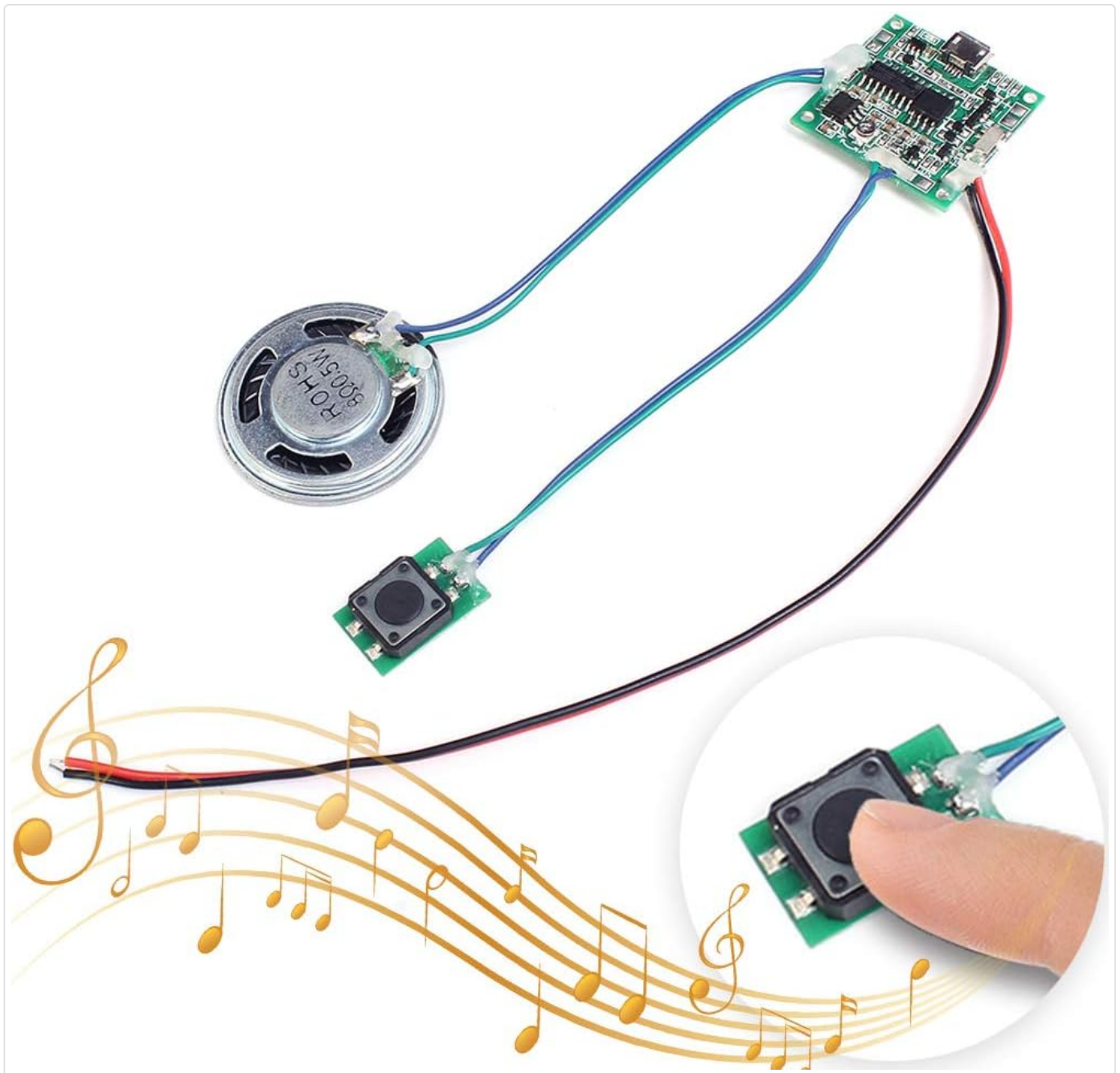
Main components of the Icstation Recordable Sound Module.
