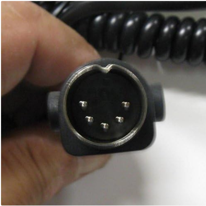
Detailed view of the round 5-pin connector of the OKIN Lift Chair Hand Control, essential for connecting to the lift chair motor.
