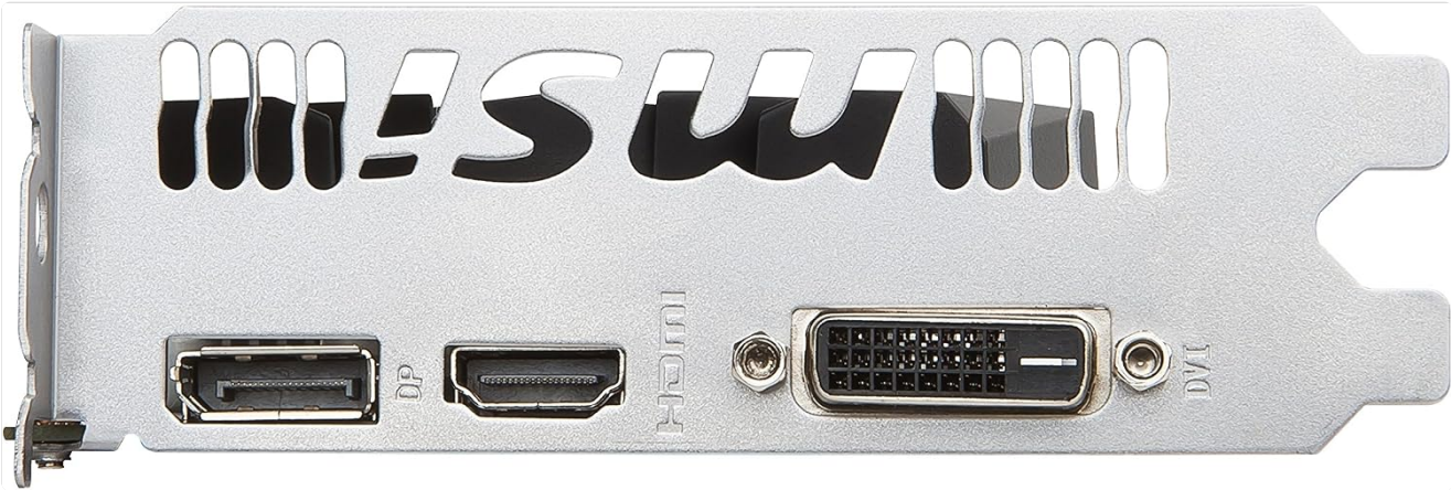
Image 4.1: Rear view of the graphics card, showing DisplayPort, HDMI, and DVI output ports for display connections.
