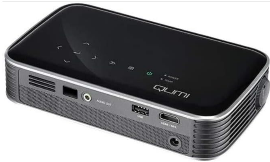
Figure 2: Side view of the Vivitek Qumi Q8-BK projector, displaying its connectivity ports. These include an audio out jack, a USB port, and an HDMI/MHL input, along with ventilation grilles.
