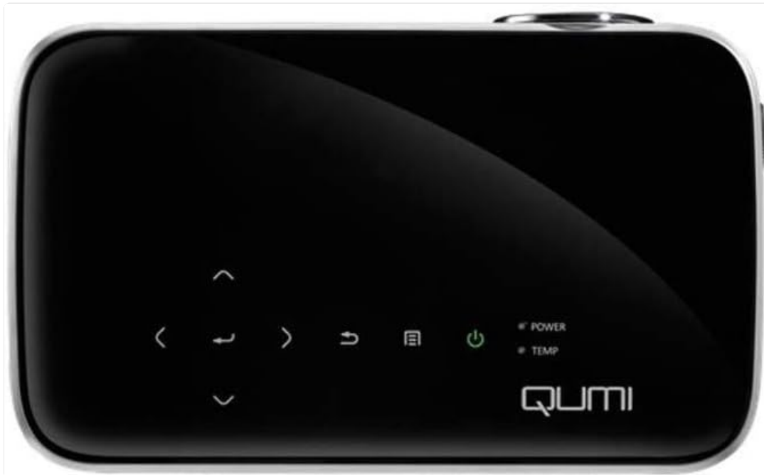
Figure 1: Top view of the Vivitek Qumi Q8-BK projector, highlighting the touch-sensitive control panel. This panel includes navigation arrows, menu access, source selection, and power buttons, along with LED indicators for power and temperature.
