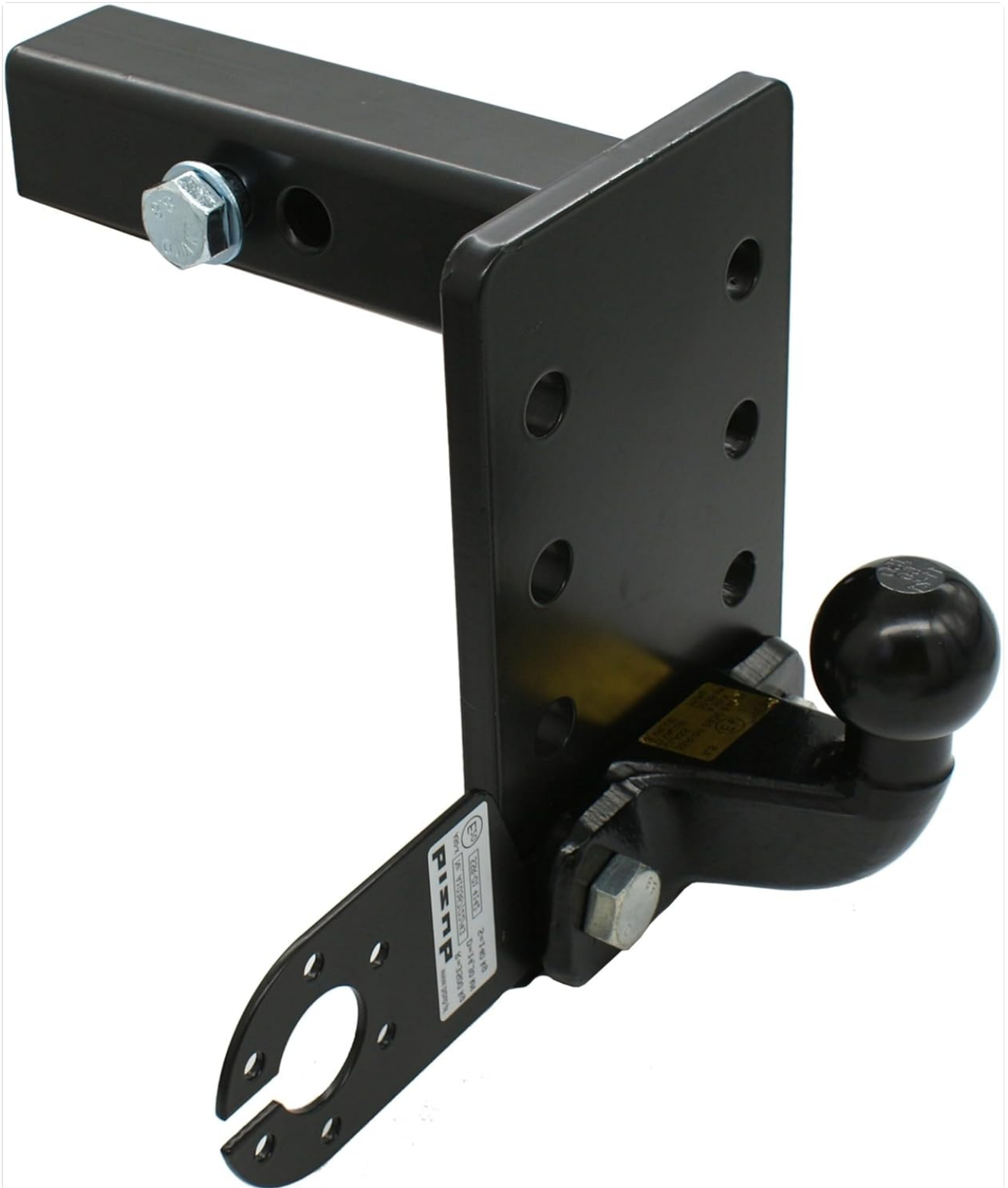
Figure 1: AHK US-Adapter Tow Hitch Device. This image displays the complete tow hitch assembly, including the 50x50mm square tube adapter, the height-adjustable mounting plate with multiple bolt holes, and the ISO 50 ball head attached. A safety pin or bolt is visible securing the adapter within the receiver. The identification plate is also visible on the side of the mounting plate.
