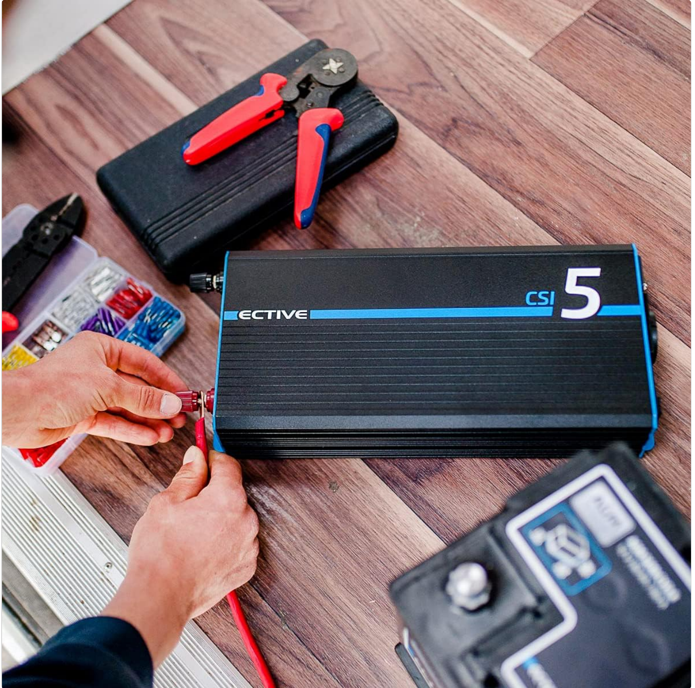
Image: An example of connecting the positive battery cable to the inverter, demonstrating the secure connection process.
