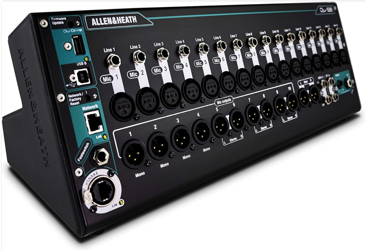
Figure 1: Front view of the Allen & Heath QU-SB, showing the 16 mic/line inputs, stereo input, and mix outputs.
