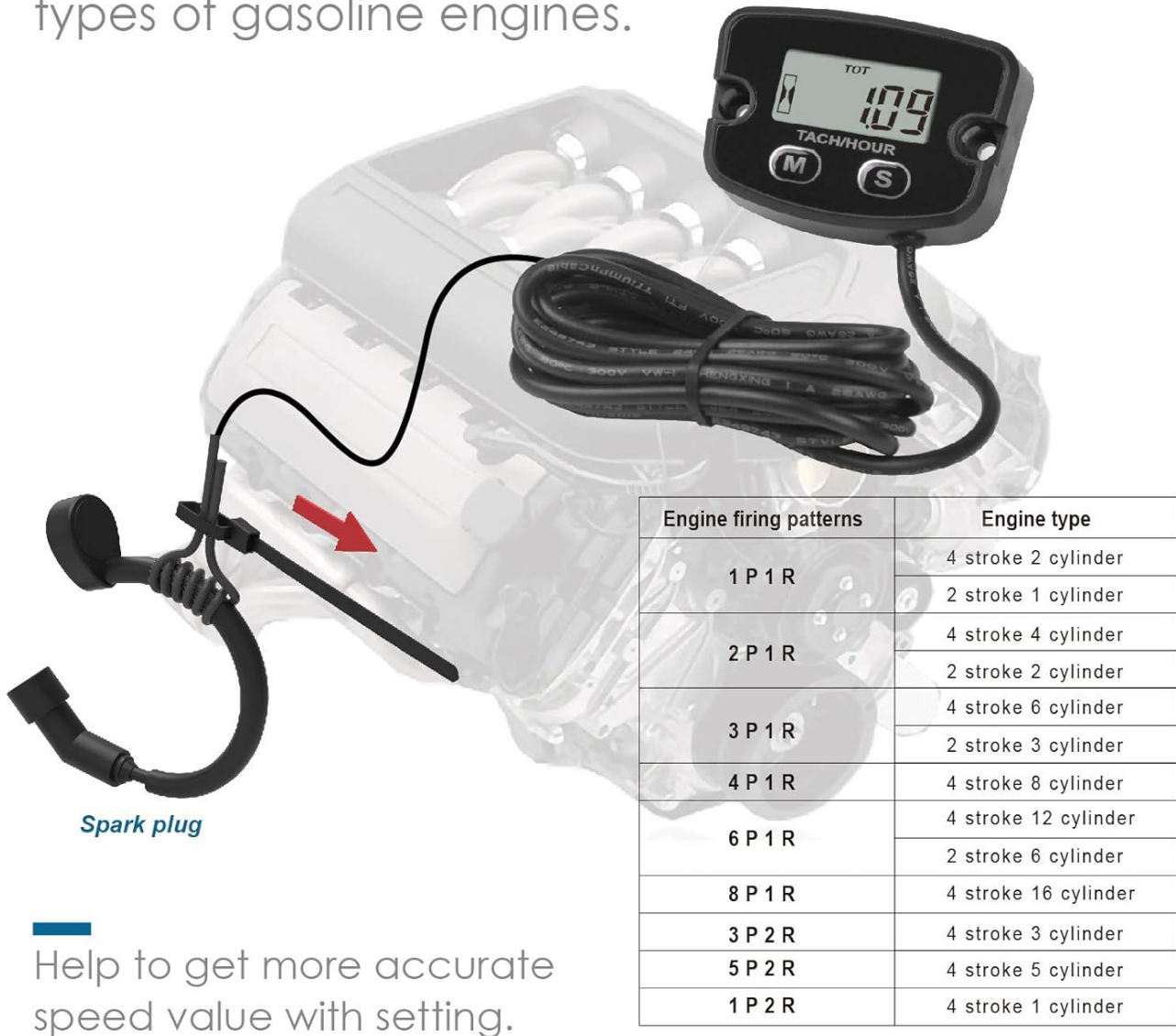
Figure 3.1: Programmable Firing Patterns. This image illustrates how the inductive wire connects to the spark plug and provides a table of common engine firing patterns and their corresponding engine types. Setting the correct pattern ensures accurate speed values.
