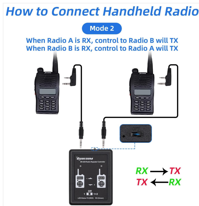
Image: A visual representation of Mode 2, showing bidirectional audio flow between Radio A and Radio B through the SR-629 controller, enabling two-way communication.
