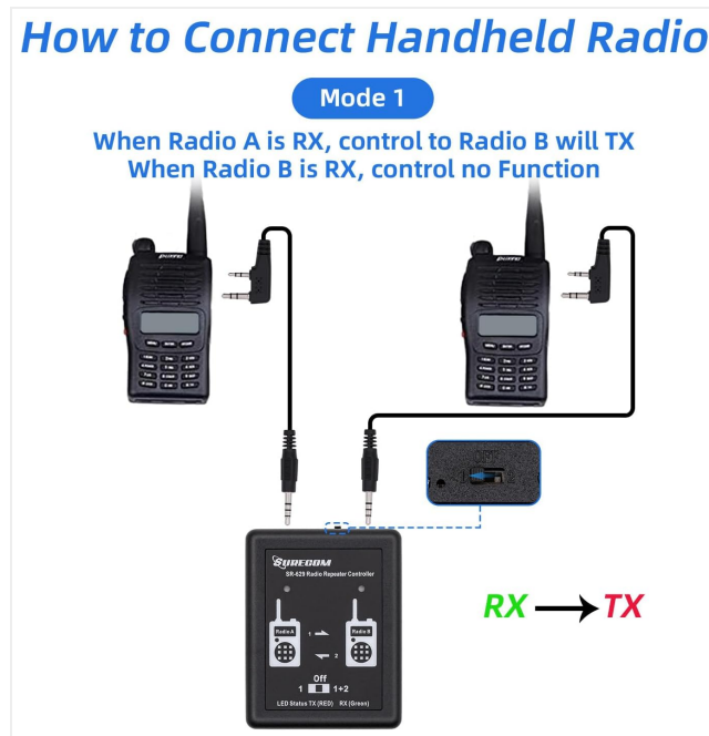
Image: A visual representation of Mode 1, showing audio flow from Radio A (Receive) to Radio B (Transmit) through the SR-629 controller.
