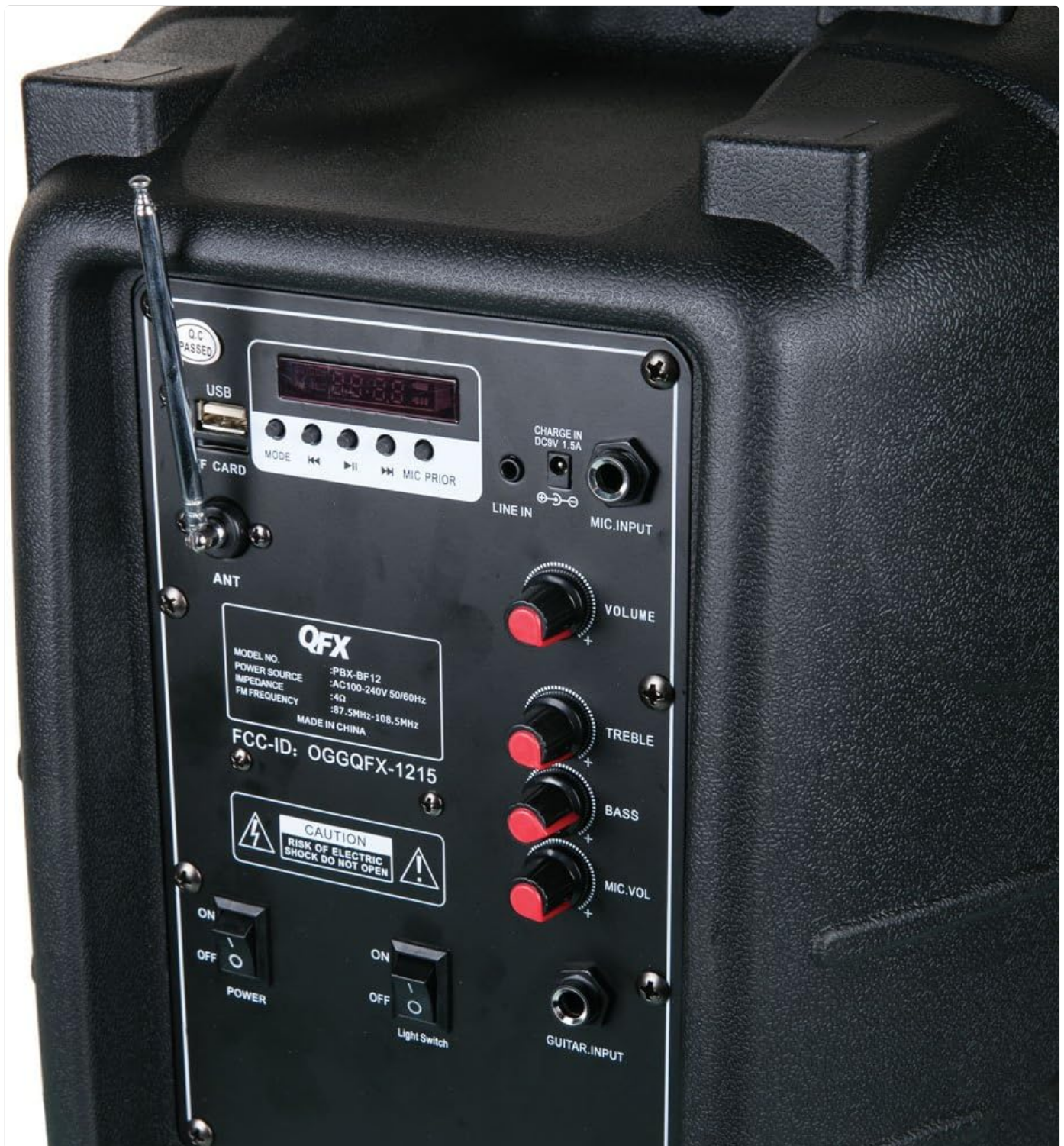
Figure 2: Rear control panel of the QFX PBX-BF12 speaker. This detailed view highlights the various inputs and controls available on the speaker's back. Key elements include the USB port, TF card slot, antenna, LED display, charging input, Line In (AUX) port, Microphone Input, Guitar Input, and control knobs for Volume, Treble, Bass, and Mic Volume. Power and Light switches are also visible.
