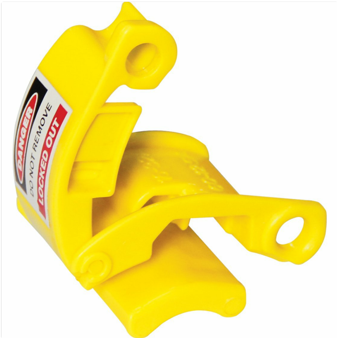
Figure 3.1: The ZING 7268 Pin and Sleeve Plug Lockout device. This yellow device is designed to encapsulate an electrical plug, preventing its insertion into a socket. It features a hinged design that closes around the plug, with a hole for a padlock shackle to secure it in place. A red and black "DANGER DO NOT REMOVE LOCKED OUT" label is visible on its side.
