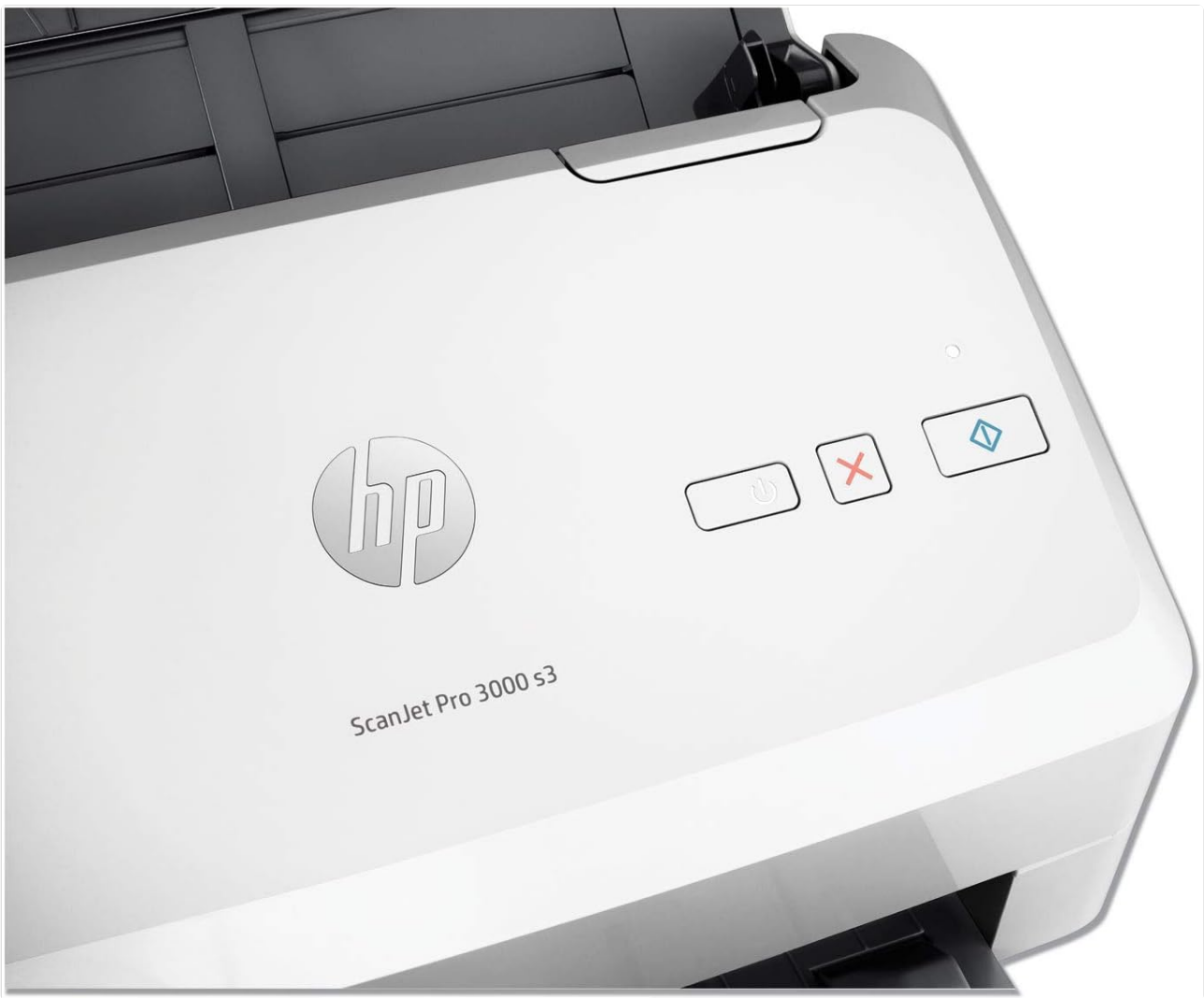
Image 3.1: Top view of the scanner showing the control panel with power, cancel, and scan buttons.
