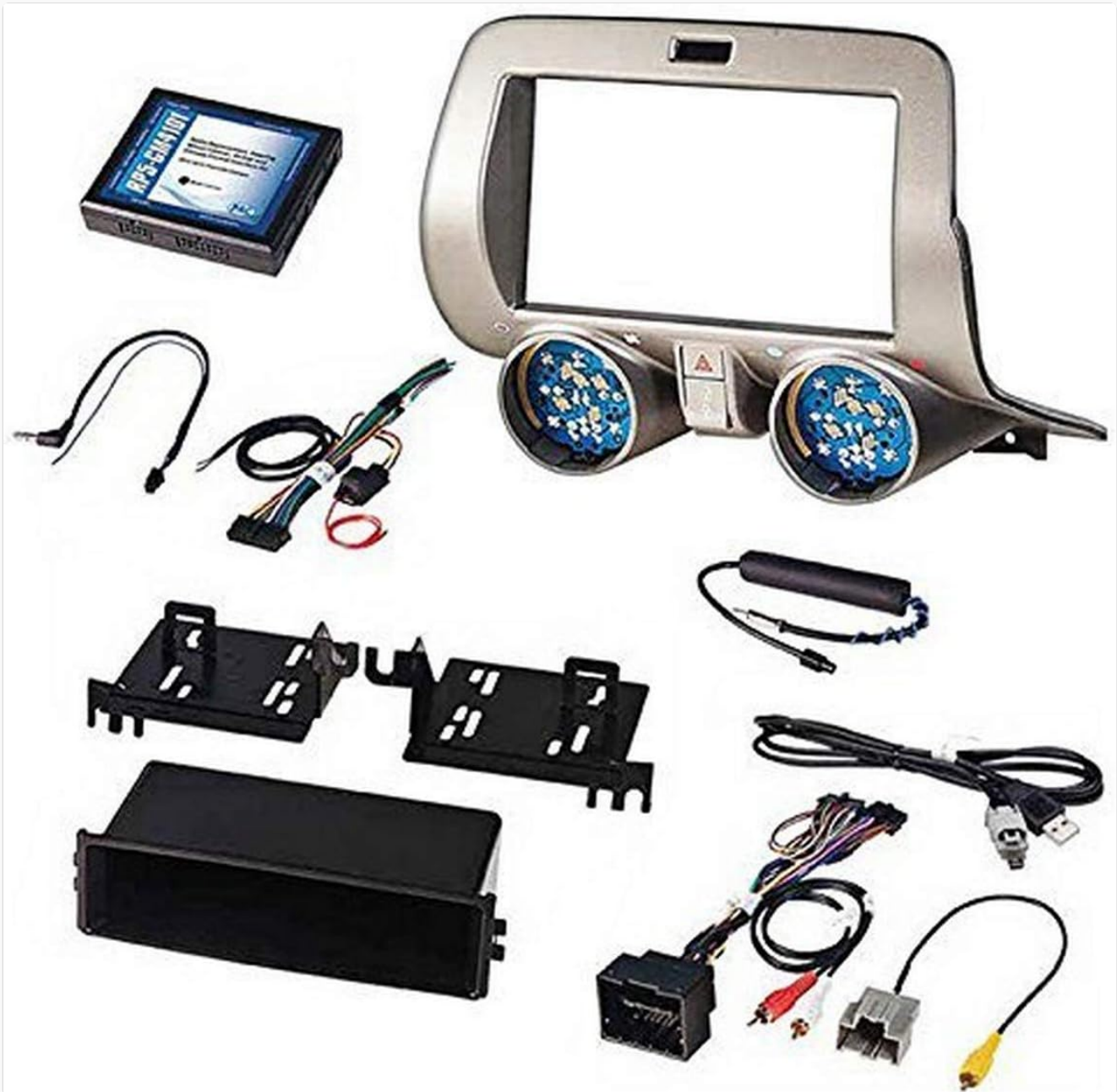
Image 1: Contents of the PAC RPK5-GM4101 kit. This image displays the main components included: the silver-colored dash kit with climate control openings, the black electronic interface module (RP5-GM4101), various wiring harnesses for power, speakers, auxiliary input, and USB, and black mounting brackets for the aftermarket radio. A single DIN pocket is also visible.
