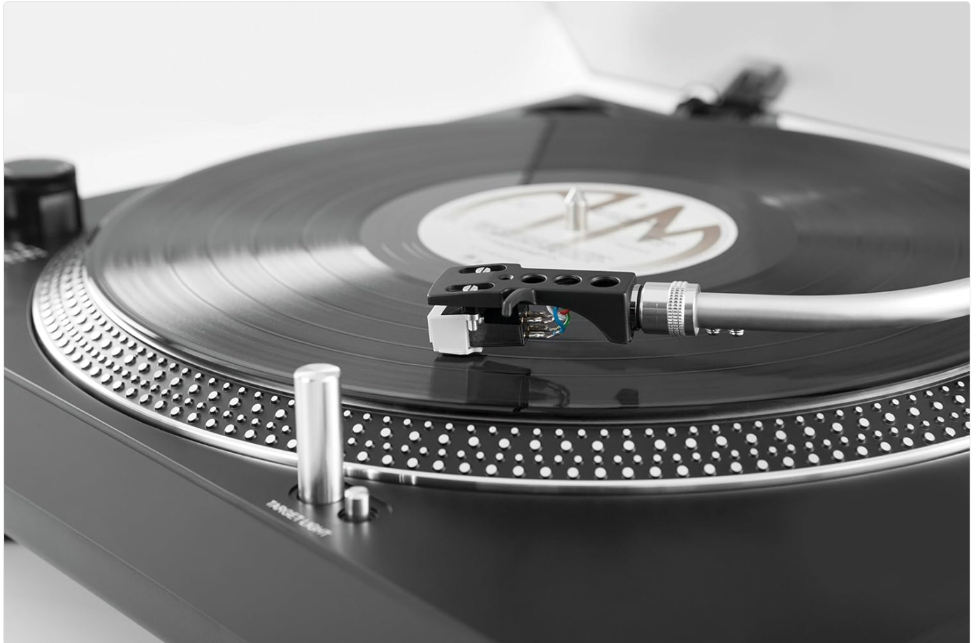
Figure 2: Detailed view of the tonearm and cartridge assembly, crucial for proper record playback.
