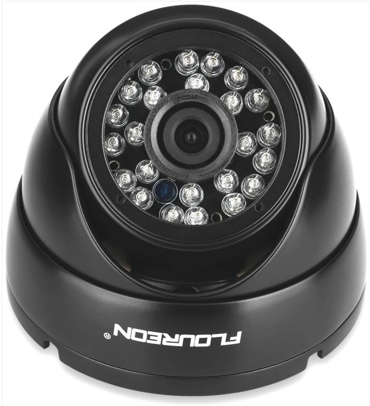
Figure 4.2: Close-up of a FLOUREON 1000TVL dome security camera with IR LEDs. A detailed view of one of the FLOUREON 1000TVL dome cameras, showcasing its robust design and integrated infrared (IR) LEDs for night vision capabilities.
