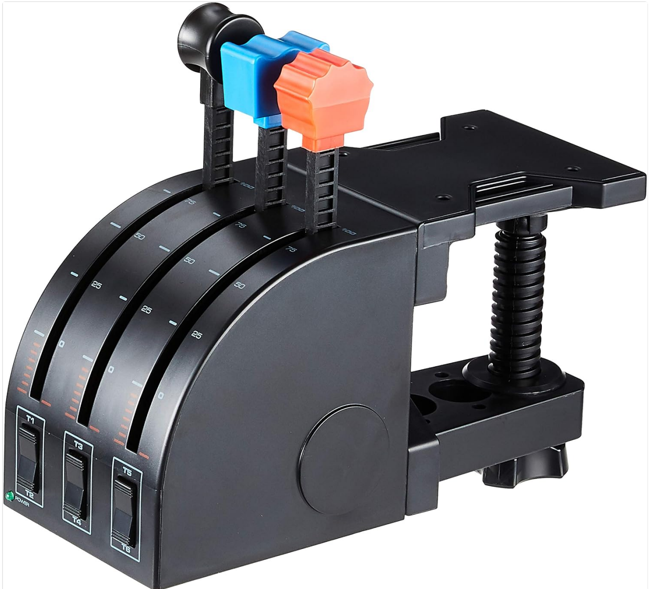
Image: A detailed view of the throttle quadrant, highlighting the three levers with numerical markings and the three two-way rocker switches labeled T1-T6.
