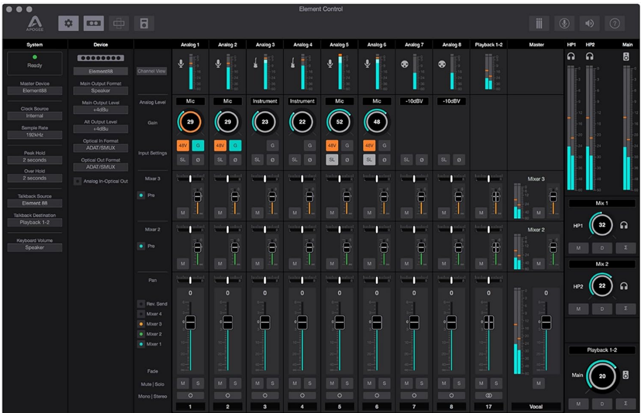
Figure 3: The Element Control software interface displayed on a computer monitor, showing virtual faders, input gain controls, output levels, and monitoring options for comprehensive hardware management.
