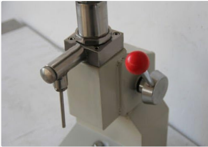
Figure 4: Close-up of the volume adjustment mechanism. This image highlights the knob or lever used to set the desired filling volume for each dispense.
