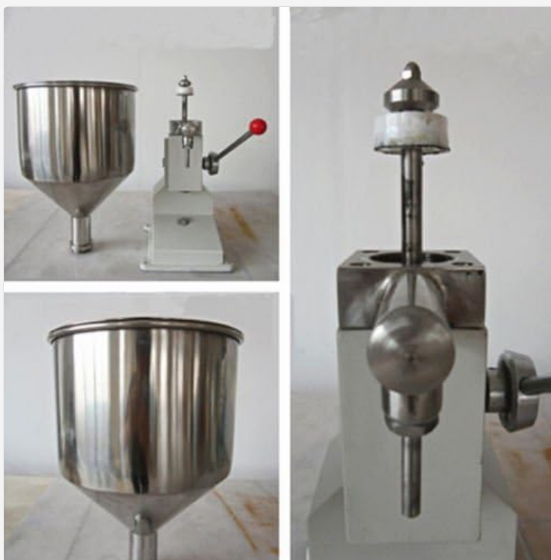
Figure 3: Disassembled components of the A03 machine. This image shows the hopper detached from the main body, illustrating how the parts fit together during assembly.
