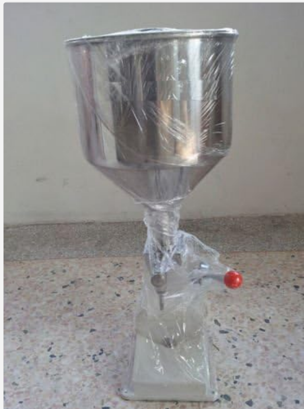
Figure 5: The A03 machine ready for operation. This image shows the machine with the hopper attached and the manual lever in position, indicating readiness for filling.
