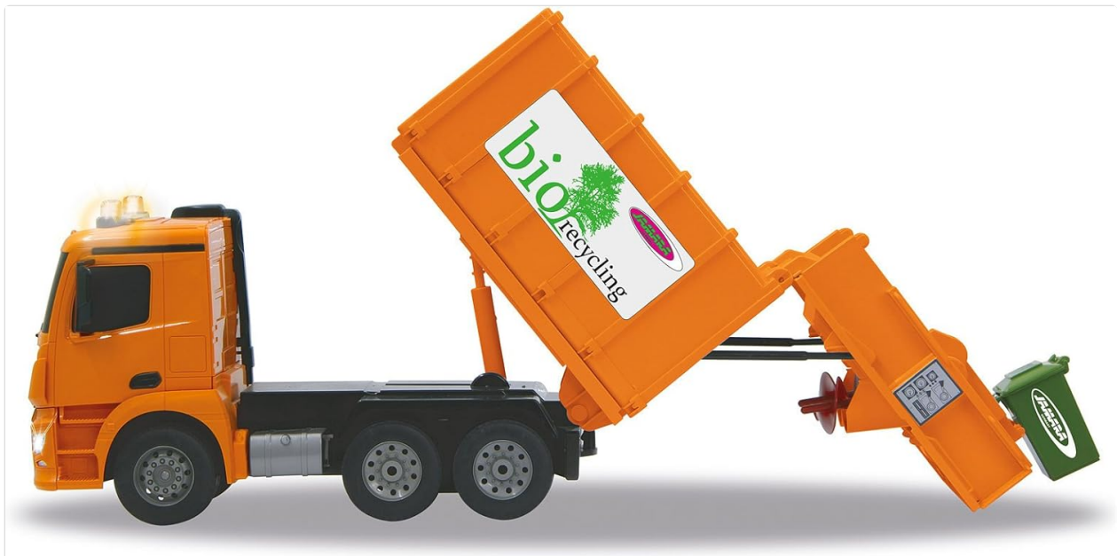
Figure 4.2: The truck's rear compartment in the tilted position for waste discharge.
