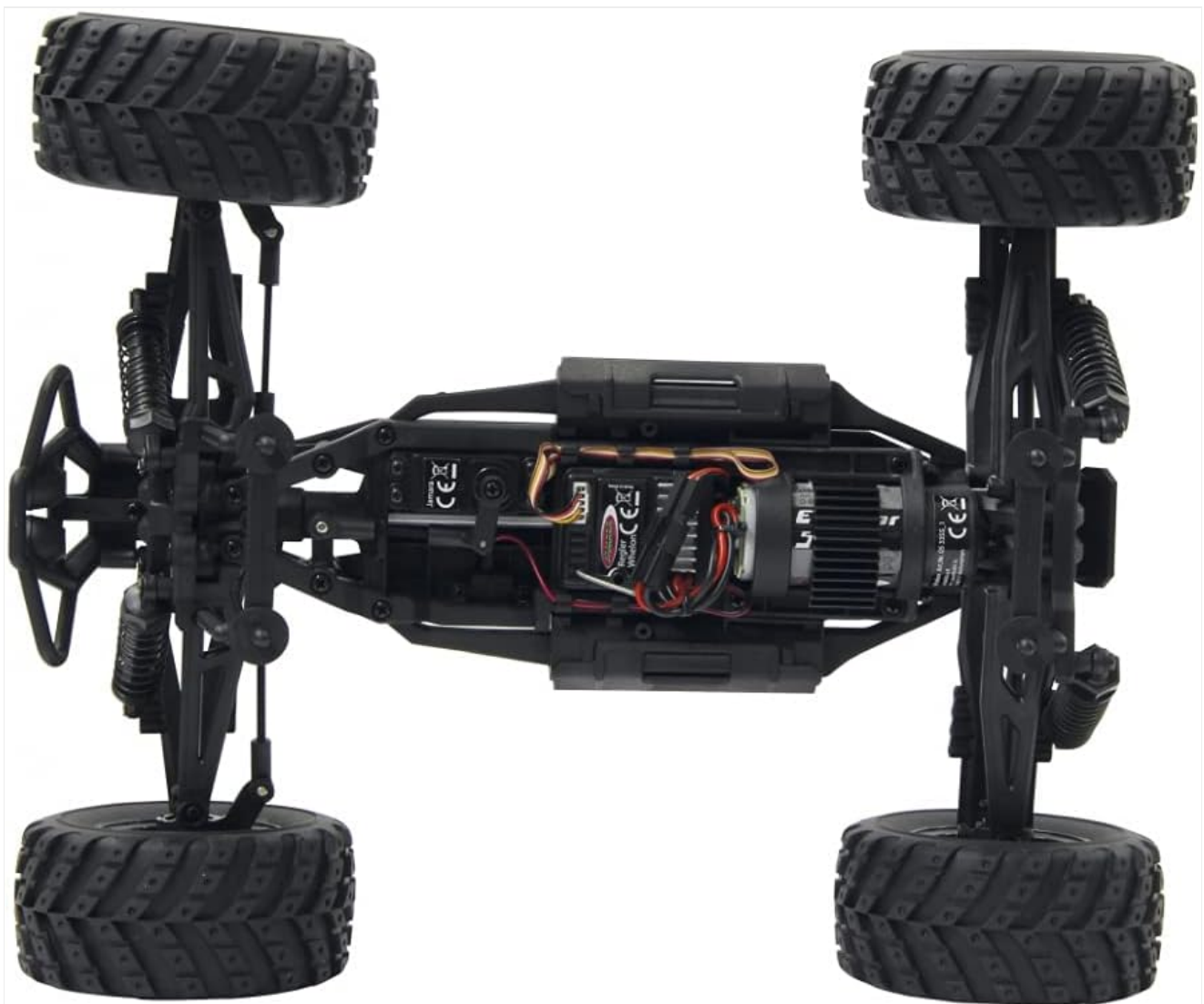
Image 4.2: Underside view of the Whelon chassis, showing the drivetrain, motor, and suspension components.
