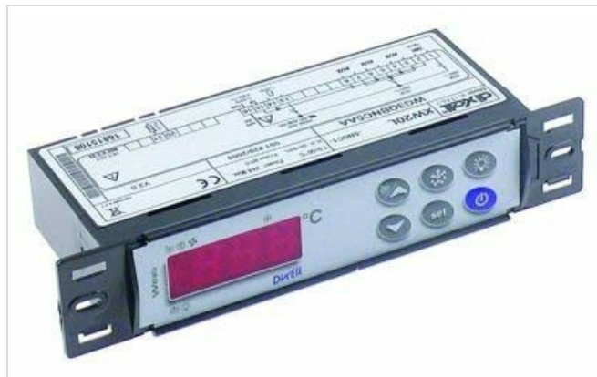
Image 1.1: Front view of the DIXELL XW60L Digital Controller, showing the red LED display and the six control buttons (up, down, set, light, defrost, power).
