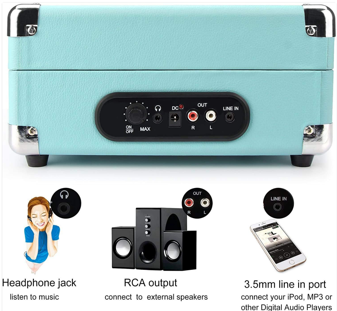
Figure 5: Visual representation of the connectivity options: headphone jack for private listening, RCA output for external speakers, and 3.5mm line-in for connecting other audio devices.
