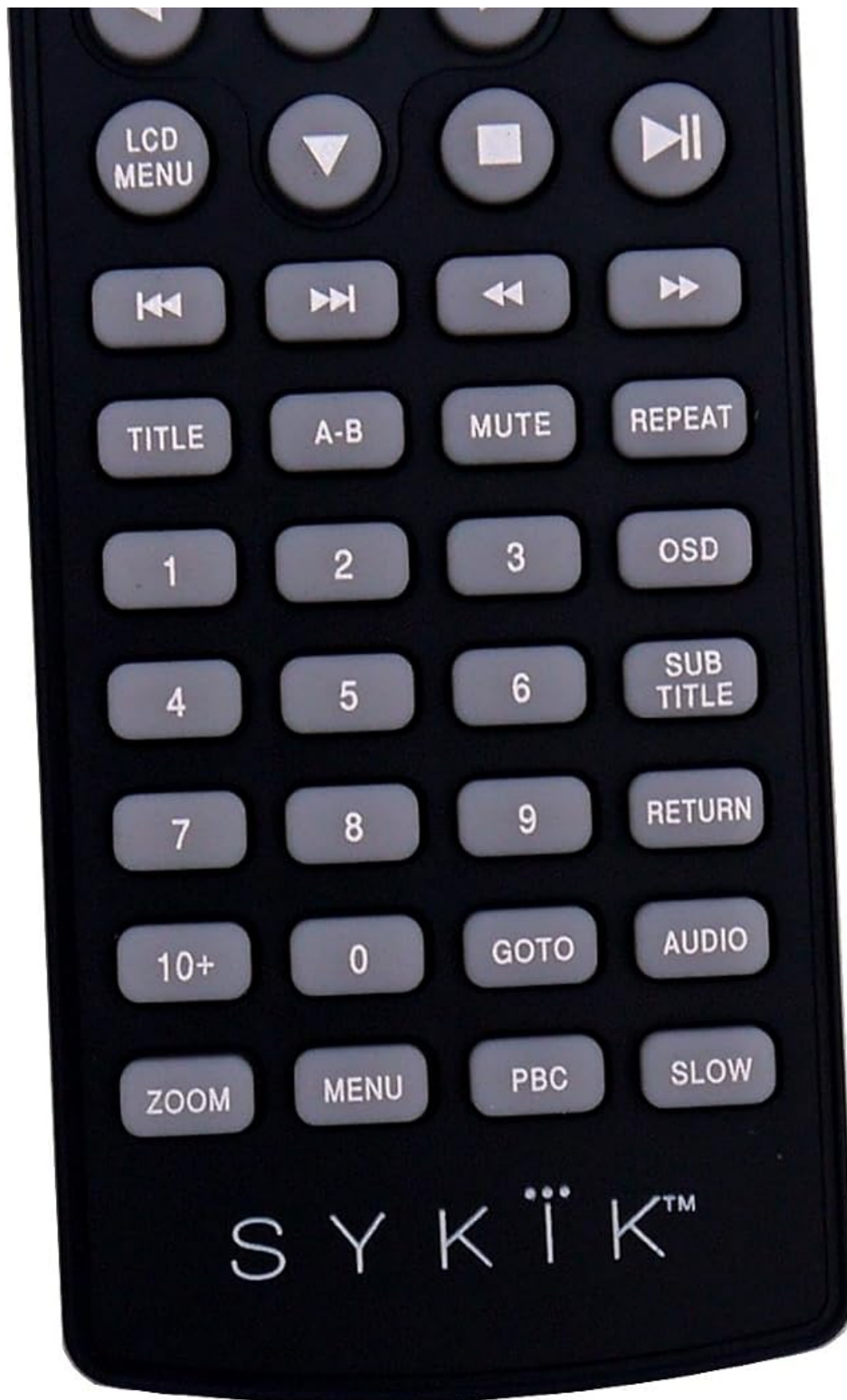
Figure 2: The remote control for the Sykik SYDVD9113TV, showing various function buttons for power, volume, mode selection, playback, and menu navigation.
