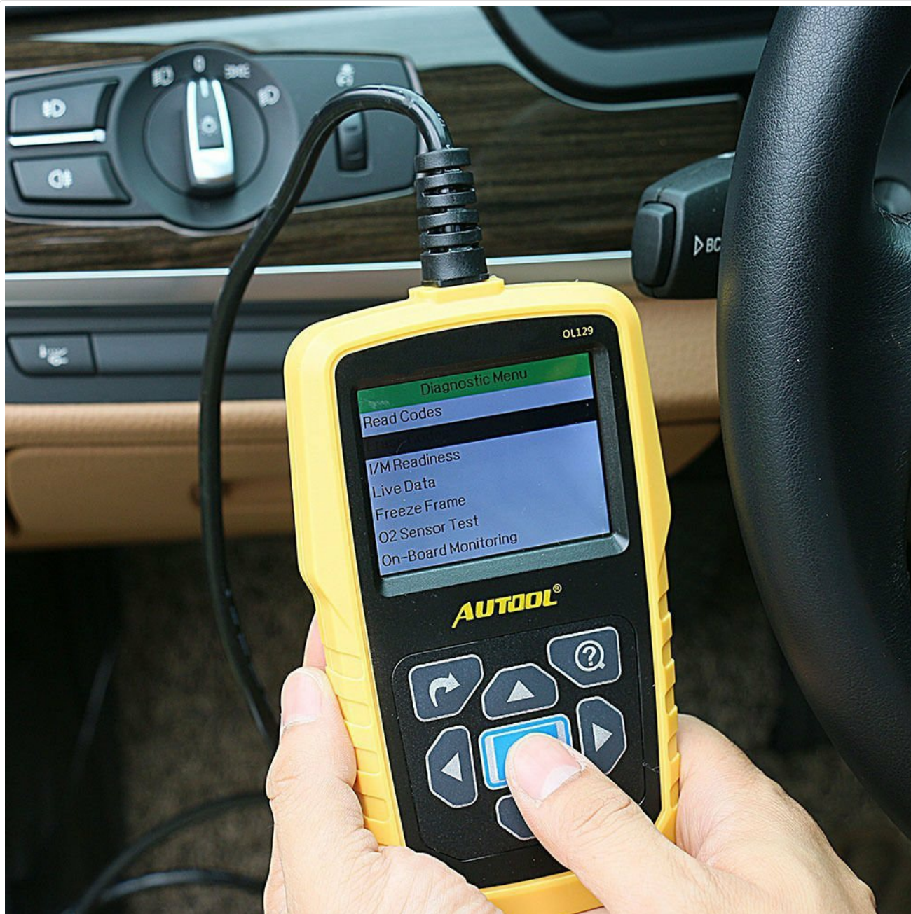
Image: The AUTOOL OL129 diagnostic tool displaying the diagnostic menu, showing options such as Read Codes, I/M Readiness, Live Data, Freeze Frame, O2 Sensor Test, and On-Board Monitoring.
