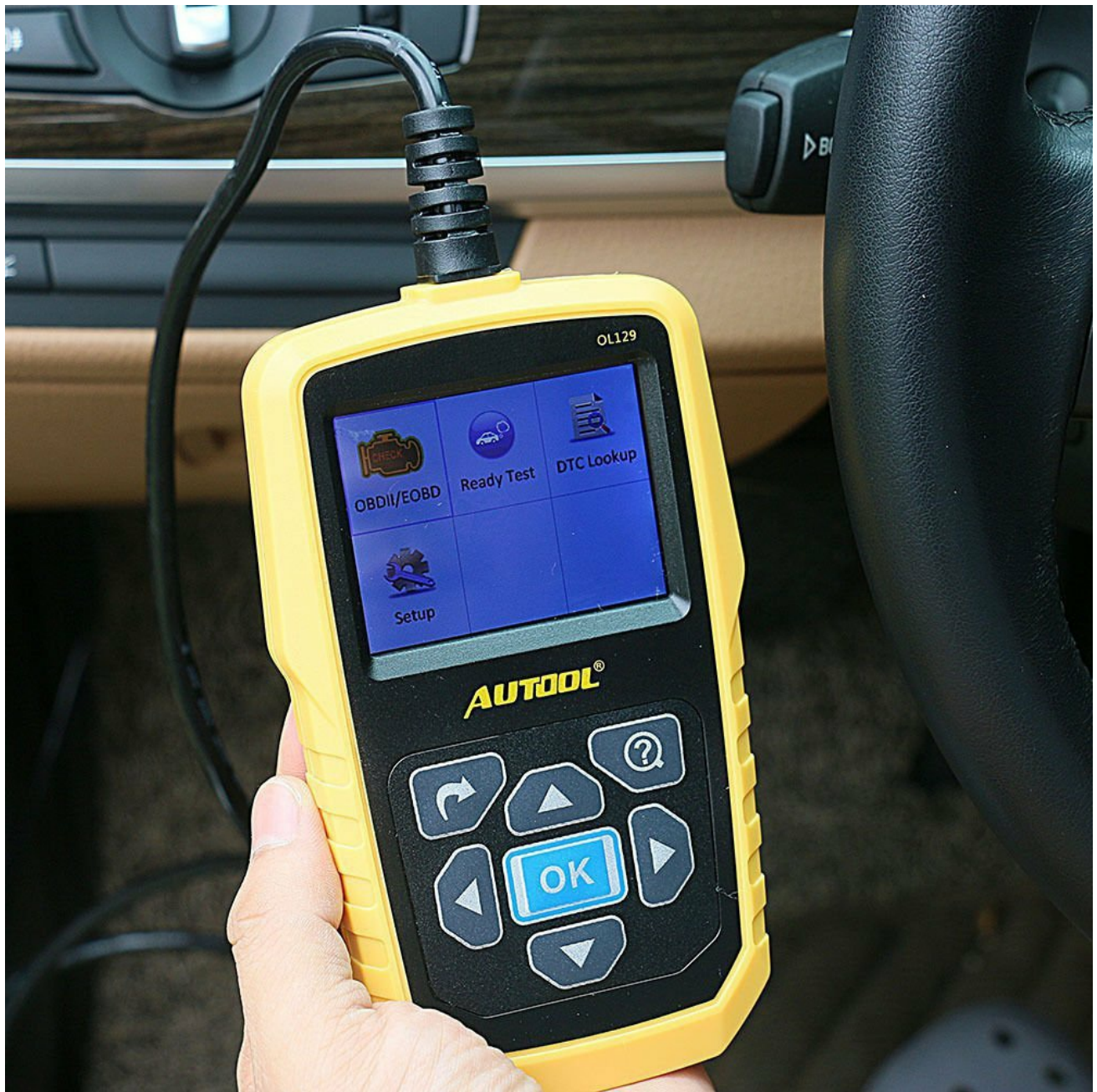
Image: The AUTOOL OL129 diagnostic tool displaying its main menu with options like OBDII/EOBD, Ready Test, DTC Lookup, and Setup.
