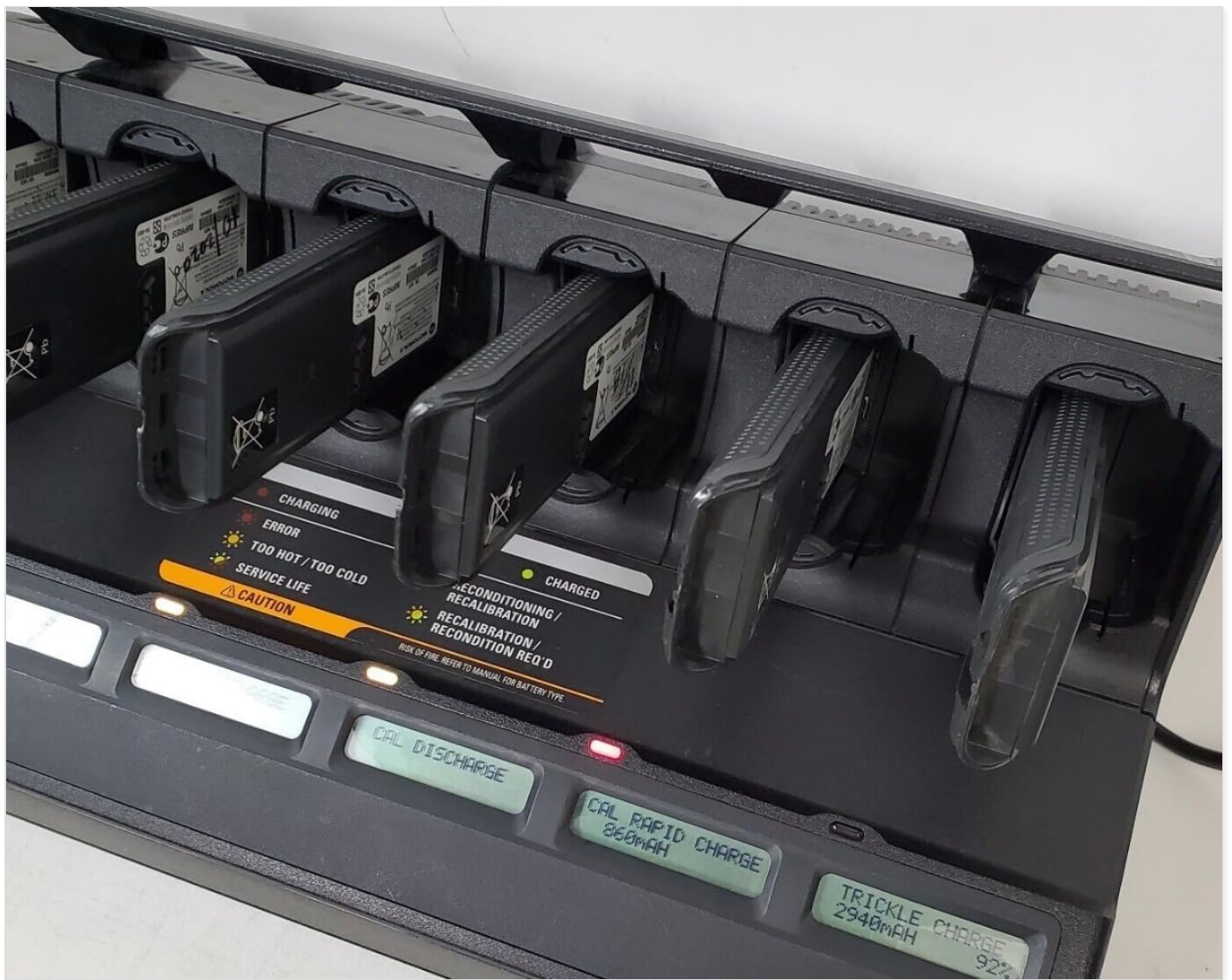
Figure 3: Batteries in Charging Bays
