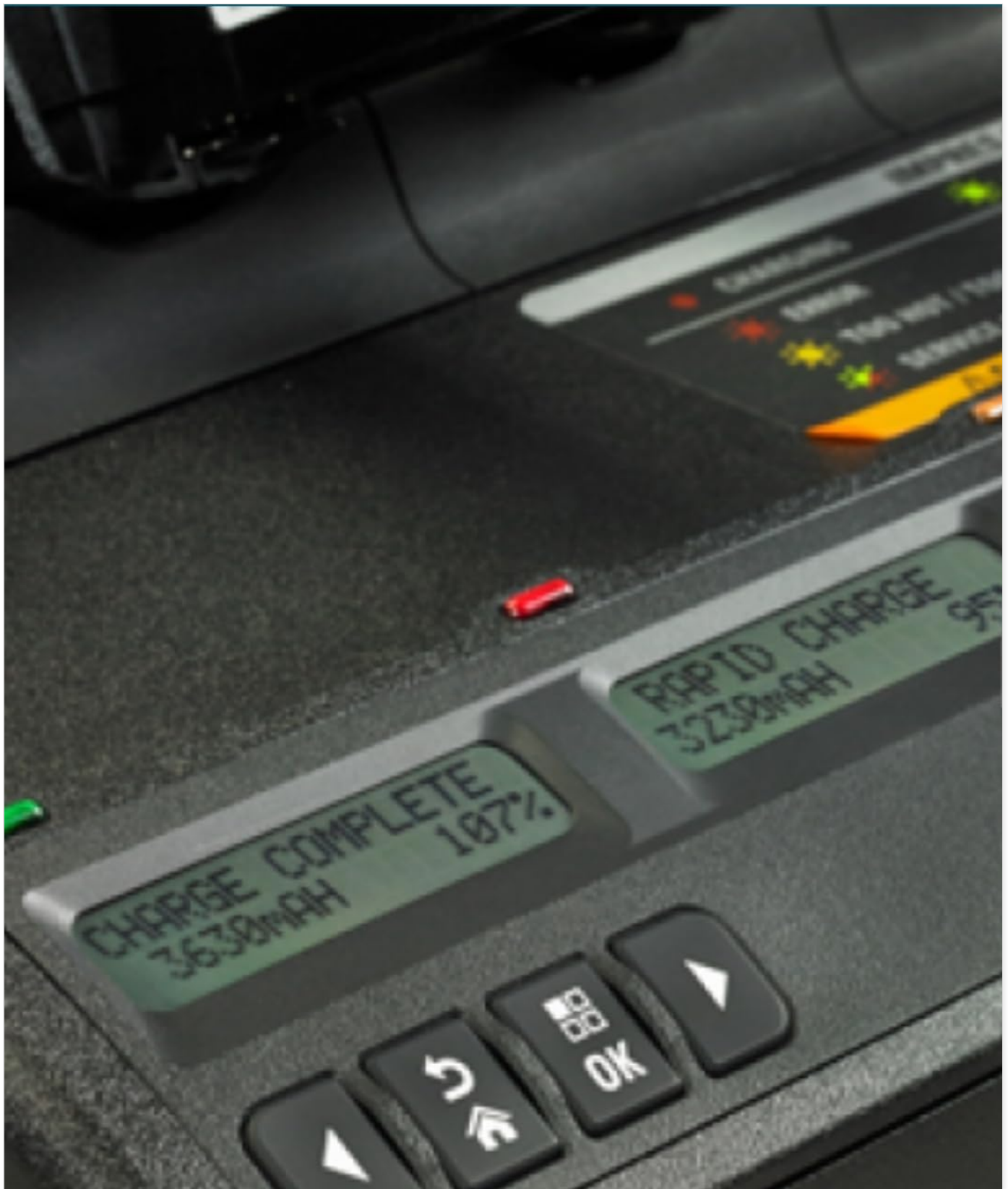
Figure 4: Charger Display Indicating Charge Complete
