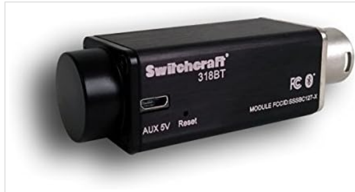
Image: A side view of the Switchcraft 318BT Bluetooth AudioStix, highlighting the micro USB port for external 5V power and a small recessed reset button. The device features a durable anodized aluminum casing.
